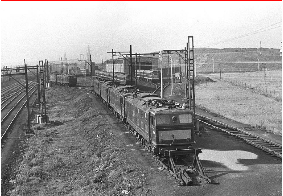
A typical 1960s scene at the depot at Wath . The depot building in the background evolved from an electric locomotive maintenance and inspection shed into a diesel inspection and fuelling facility after the London Midland Region took over responsibility for electric locomotive maintenance in 1958. Electric locomotives though continued to be stabled at Wath. J Leaf/Colour-Rail 30319
