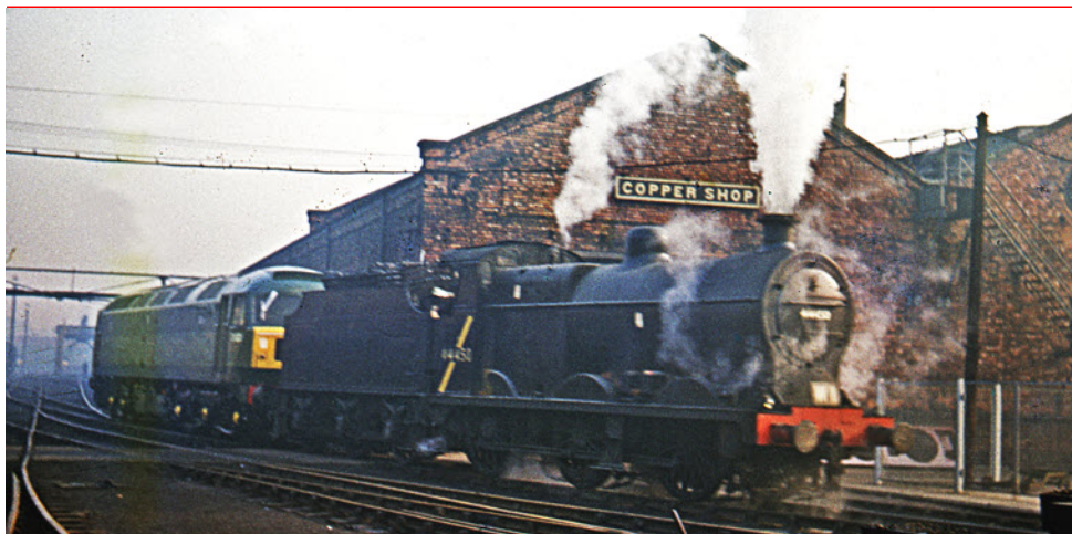
Crewe Works shunter ex-LMS Class 4F 0-6-0 No.44450 is pictured on November 1st, 1964 outside the 'Copper Shop' moving a newly Crewe-built Type 4 Brush diesel locomotive. N Joseph/Colour-Rail 316003
